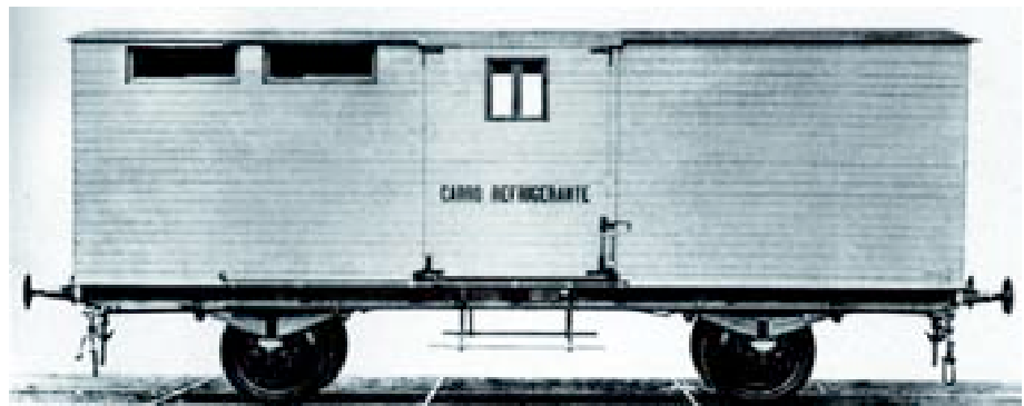
Figure 2.2 - 1906, the first refrigerated coach for the transport of perishables
